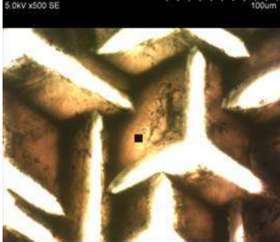
Self-organized materials - manufactured via directional solidification of eutectics
